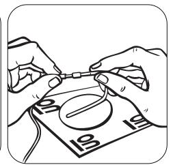
Hold the pin connector while disconnecting or inserting pin.
