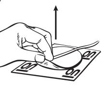
Remove an electrode by lifting its edge.
