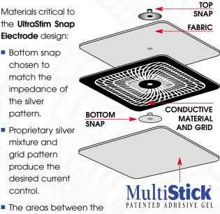
lines of the silver grid pattern are calculated to fill in gaps creating efficient current control.
