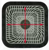
biting and stinging, resulting in stimulation comfort. Conventional electrodes with flood coated silver to the edges provide current distribution that may be amplified at the edges and usually causes edge biting and stinging.
